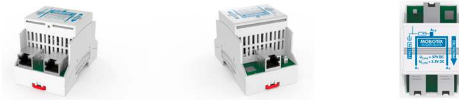
Connections on the Mx-A-SPA-HR (two views of device): 2 RJ45 to the switch (for two PoE devices) and 1 RJ45 (to the patch panel)
